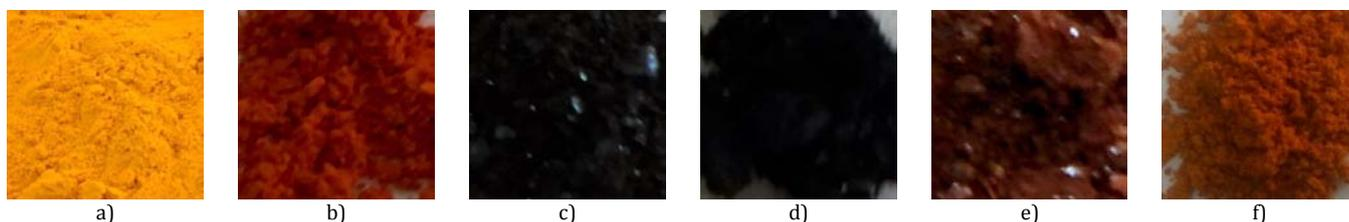
Fig. 1: The physical appearance of curcumin complexes a) curcumin, b) Cur-Zn, c) Cur-Cu, d) Cur-Fe, e) Cur-Mn, f) Cur-Mg
