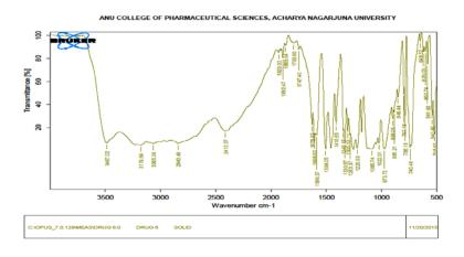
Fig. 3: IR Spectrum for carvedilol phosphate
