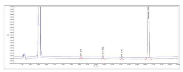
Fig. 3: HPLC chromatogram of sample spiked with impurities (DP-1, DP-2 and DP-3)
