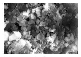
Fig. 6: SEM Micrograph of biosynthesized titania nanoparticles by *Lactobacillus* sp
