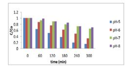
Fig. 9: The effect of pH on dye decolourization by titania nanoparticles
