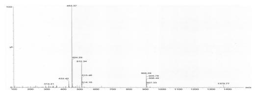
Fig. 3C: Mass spectrum of impurity at RT 7.230 min
