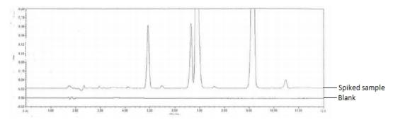
Fig. 4: Overlay chromatogram of blank and fluticasone propionate nasal solution
