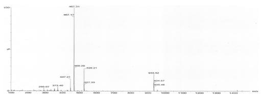
Fig. 3D: Mass spectrum of impurity at RT 8.948 min
