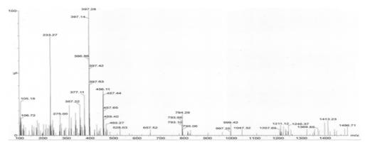
Fig. 3A: Mass spectrum of impurity at RT  $5.043\ min$
