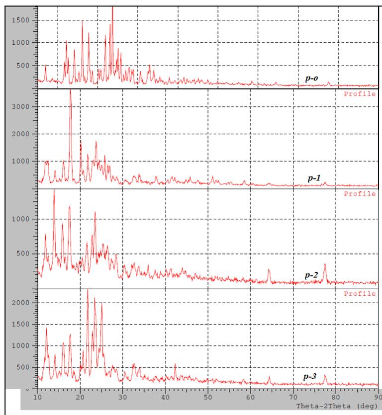
Fig. 3: X-ray patterns for Prulifloxacin (P-0) and its polymorphs (P-1, P-2, P-3)
