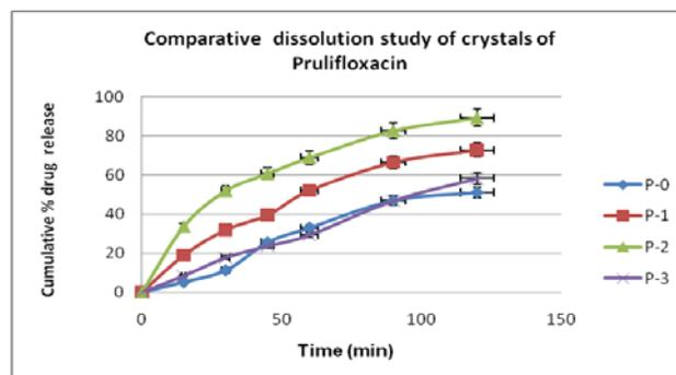
Fig. 6: Graph for comparative dissolution study data (P-0 =amorphous form, P-1 = polymorph 1, P-2 = polymorph 2, P-3 = polymorph-3) (\*n=4)
