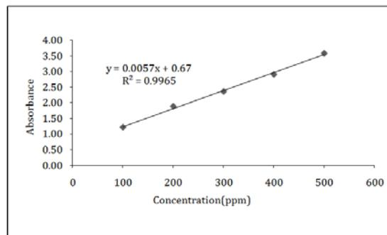
**Fig. 1: Calibration curve for Sodium benzoate at 228 nm**
