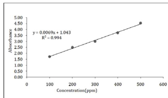
**Fig. 2: Calibration curve for potassium sorbate at 250 nm**
