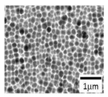
Fig. 3: SEM image of the ziprasodone (ZIP) nanocrystals
