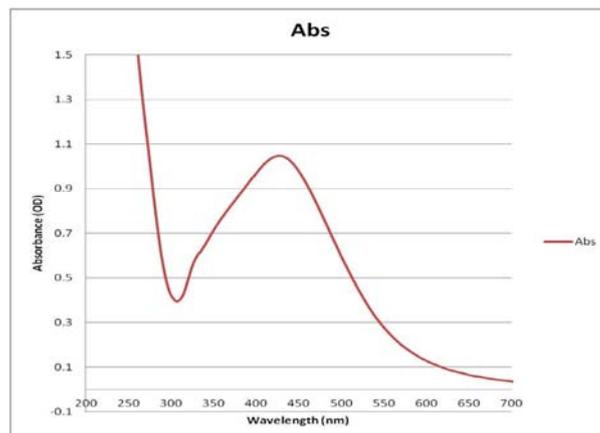
Fig. 3: UV-Visible absorption spectrum of AgNPs synthesized from *S. samarangense* leaf extract
