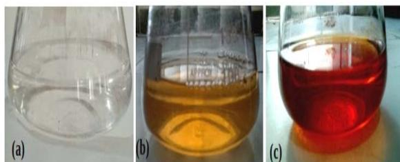
Fig. 2: (a)  $\text{AgNO}_3$  solution (control) (b) *S. samarangense* (Java Apple) leaf extract (c) Synthesized AgNPs
