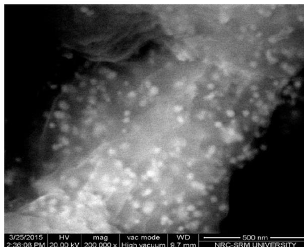
Fig. 5: FESEM showing spherical AgNPs synthesized from *S. samarangense* aqueous leaf extract
