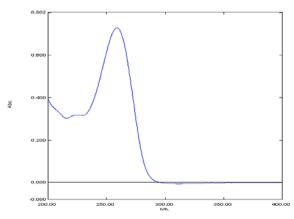
Fig. 3: UV spectrum of standard Diloxanide furoate
