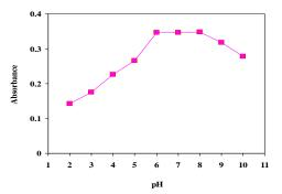
Fig. 2: Effect of pH on the absorbance after CPE. Conditions: Ni(II), 200 ng/ml; BTAO, (1.0 × 10<sup>-4</sup> mol/l) and Triton X-114, 0.2% (v/v). Other experimental conditions are described under procedures
