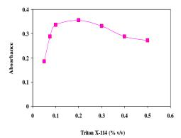
Fig. 4: Effect of Triton X-114 concentration on the absorbance after CPE. Conditions: Ni(II), 200 ng/ml; BTAO, (1.0 × 10<sup>-4</sup> mol/l) and pH 7.0. Other experimental conditions are described under procedures
