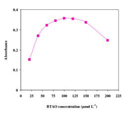
Fig. 3: Effect of BTAO concentration on the absorbance after CPE. Conditions: Ni(II), 200 ng/ml; Triton X-114, 0.2% (v/v) and pH 7.0. Other experimental conditions are described under procedures
