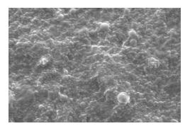
Fig. 3: Particle surface morphology of Camptothecin loaded polymeric nanoparticles prepared using FESEM
