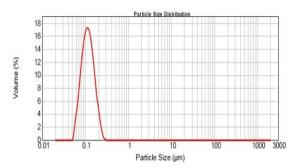
Fig. 1: Particle size spectrum of Camptothecin loaded polymeric nanoparticles prepared using sonication approach
