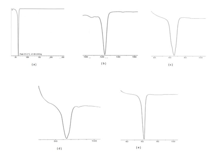
Fig. 1: DSC thermograms of: (a) Softisan® 154, (b): Phospholipon® 90H, (c): SRMS 1:1, (d): SRMS 2:1, (e): SRMS 1:2.
